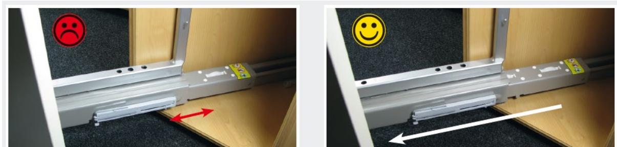
This will result in an automatic self-adjustment of the cabinet and it will close completely.
