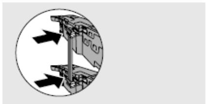
Two drive units that need to eject at the same time must be connected via the synchronisation cable.
