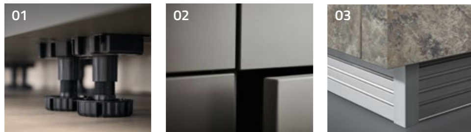
01. The positioning of the plinth feet can be adjusted if required. Height adjustment +18/-10 mm. 02. Particularly narrow joints. 03. Lamella base – ventilation for built-in devices, for example hob extractors. Aluminium or black.
